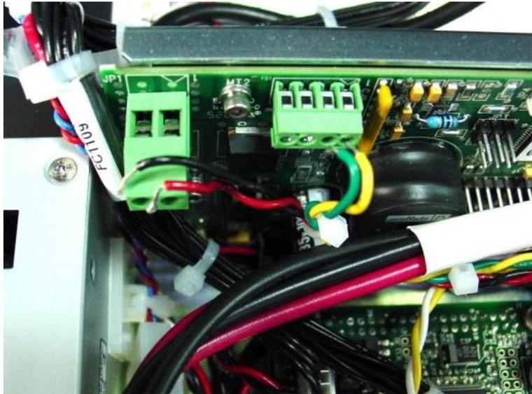
Figure 3: Remove Wires from JP1 and JP5
